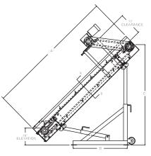
**TAKE-UP:** Screw type unit at tail pulley provides 12" belt take-up.
